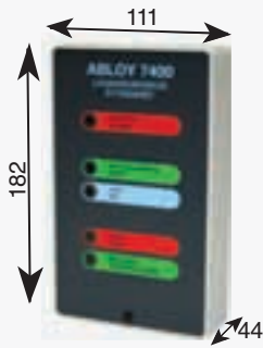
Control unit ABLOY® 7400 • Supply voltage 230 VAC • Output voltage 24VDC • Max. output current 300 mA
