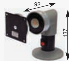
Wall magnets ABLOY® 7438, 7439 • Operating voltage 24VDC • Normal current 16mA • Hold open force 500 N
